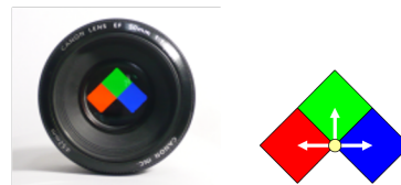
Figure 1: Color-Filter aperture set-up and orientation in a DSLR Lens.
