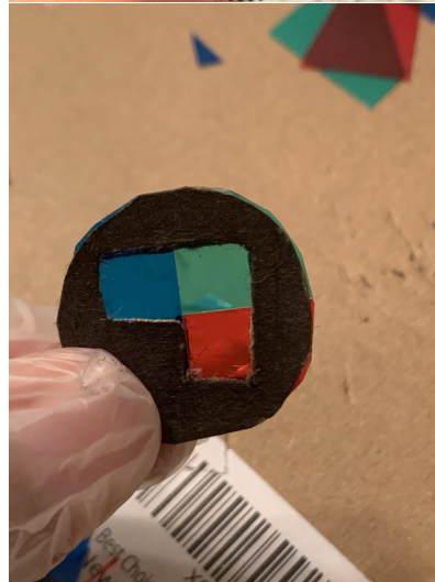
Figure 14: Construction of the Color-Filtered Aperture
